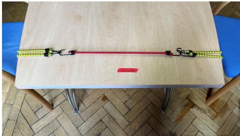
Figure 1 – The launch mechanism used to slide the pucks.
