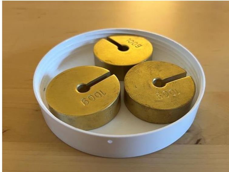
Figure 2 – A puck loaded with 3 x 100g masses.
