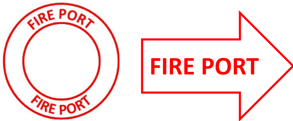
Figure 3: Fire Port location markings
