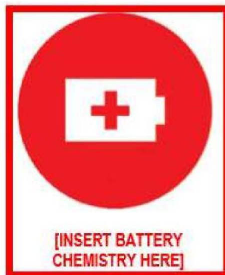
Figure 4: Battery Chemistry marking
