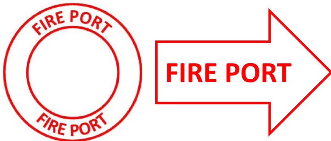
Figure 6: Fire Port marking
