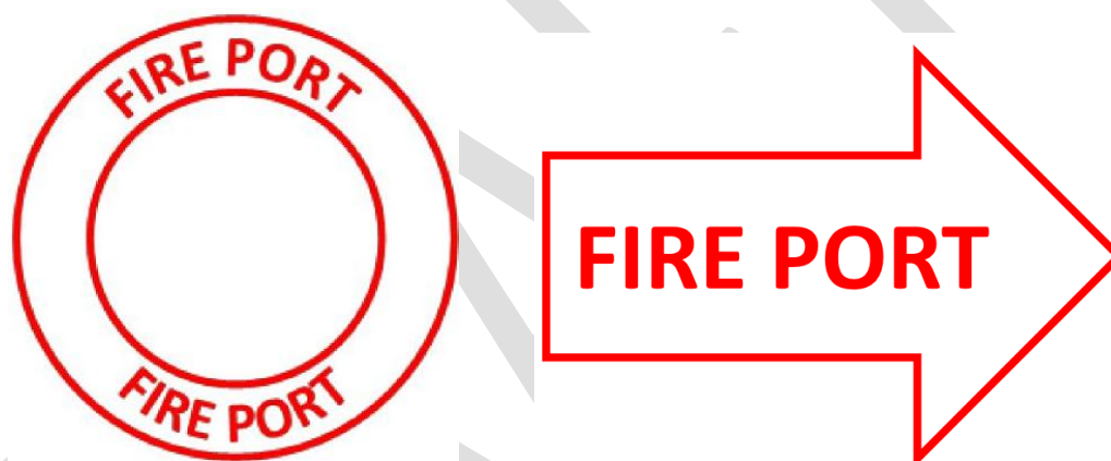
Figure 3: Fire Port location markings
