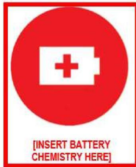
Figure 4: Battery Chemistry marking
