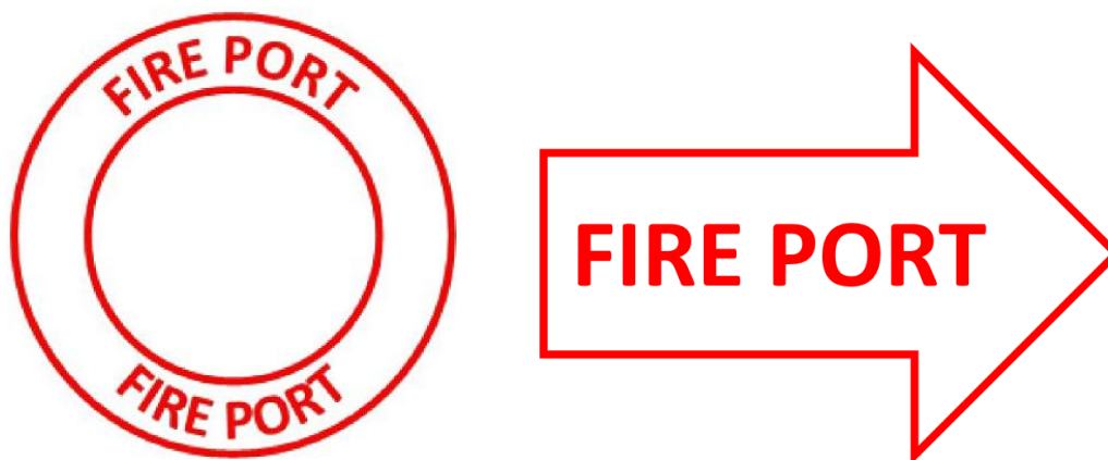
Figure 3: Fire Port location markings
